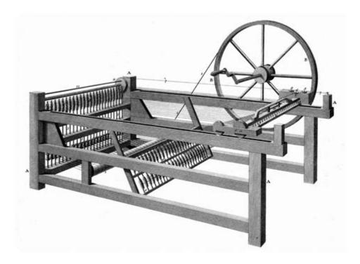
**The spinning jenny** was an innovative textile device invented in the late 18th century that revolutionized the production of yarn. Patented by James Hargreaves in 1770, the spinning jenny played a pivotal role in the Industrial Revolution, significantly increasing the efficiency of textile manufacturing. This article explores the history, mechanics, and impact of the spinning jenny on the textile industry and society at large.
