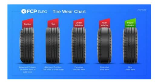
Wear on tires guide is an essential topic for vehicle owners, as it directly impacts safety, performance, and cost-effectiveness. Understanding tire wear can help you extend the lifespan of your tires, improve fuel efficiency, and enhance overall driving safety. This guide will provide insights into the types of tire wear, the factors that contribute to wear, and tips for maintaining your tires effectively.
