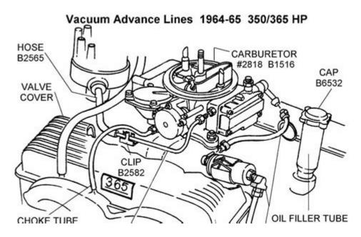
Vacuum line diagram for Chevy 350 engines is an essential tool for anyone looking to maintain or restore these classic powerhouses. Understanding the vacuum system in a Chevy 350 engine can significantly impact performance, fuel efficiency, and overall drivability. This article will delve into the intricacies of the vacuum line diagram, its importance, common configurations, troubleshooting tips, and more, ensuring you have a comprehensive understanding of this crucial component of your vehicle.
