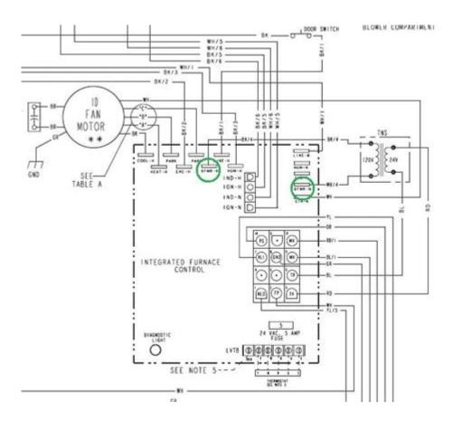
Trane air handler wiring diagram is an essential component for understanding how to install, troubleshoot, and maintain Trane air handlers effectively. Air handlers are critical for the proper functioning of HVAC systems, facilitating the distribution of conditioned air throughout residential and commercial spaces. This article will provide an in-depth look at the wiring diagrams of Trane air handlers, the components involved, and best practices for working with these systems.
