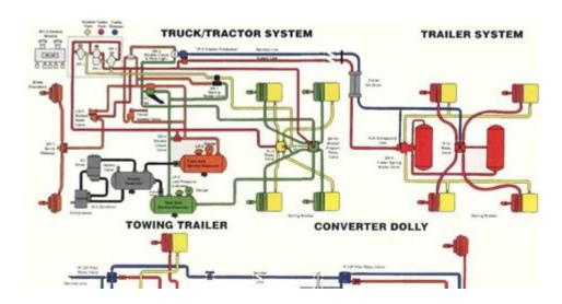
Truck air brake diagram is an essential component of understanding how heavy-duty trucks and commercial vehicles operate. Air brakes are crucial for the safe operation of trucks, given their substantial weight and the need for effective stopping power. In this article, we will delve into the intricacies of air brake systems, their components, how they work, and the importance of understanding a truck air brake diagram for maintenance and safety purposes.
