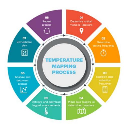
Temperature mapping validation protocol is a critical process in various industries, particularly in pharmaceuticals, biotechnology, and food production, where maintaining specific temperature ranges is essential for product integrity and safety. This article delves into the intricacies of temperature mapping validation protocols, their importance, methodologies, and best practices, ensuring compliance with regulatory standards and safeguarding the quality of sensitive products.
