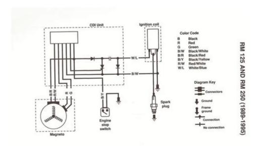
**Suzuki 12 Pin CDI Wiring Diagram** is a crucial component for any motorcycle or ATV enthusiast looking to understand the electrical systems of their vehicles. The Capacitor Discharge Ignition (CDI) system is essential for controlling the timing and firing of the engine. In this comprehensive guide, we will delve into the intricacies of the Suzuki 12 pin CDI wiring diagram, exploring its importance, the components involved, and how to troubleshoot common issues.
