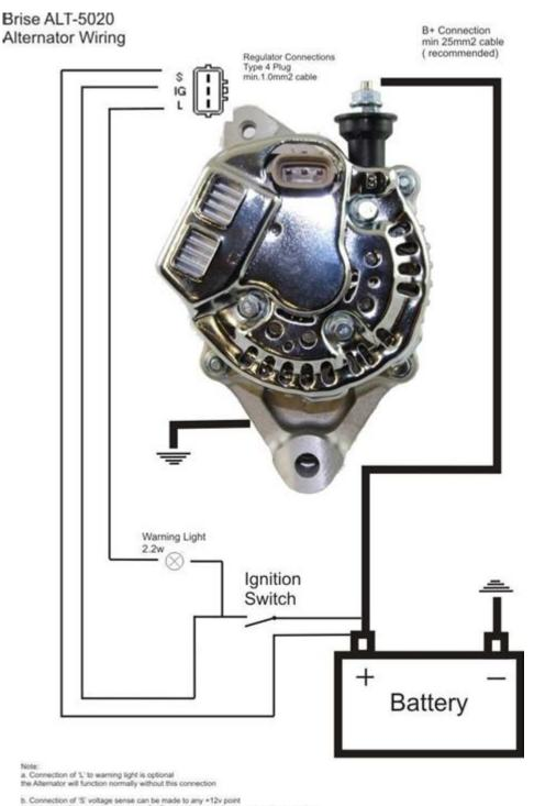
b. Connection of 'S' voltage sense can be made to any +12v point i.e. linked to 'IG' terminal or Atternator B+ Terminal however for accurate voltage sensing connection direct to Battery + terminal is preferred.
