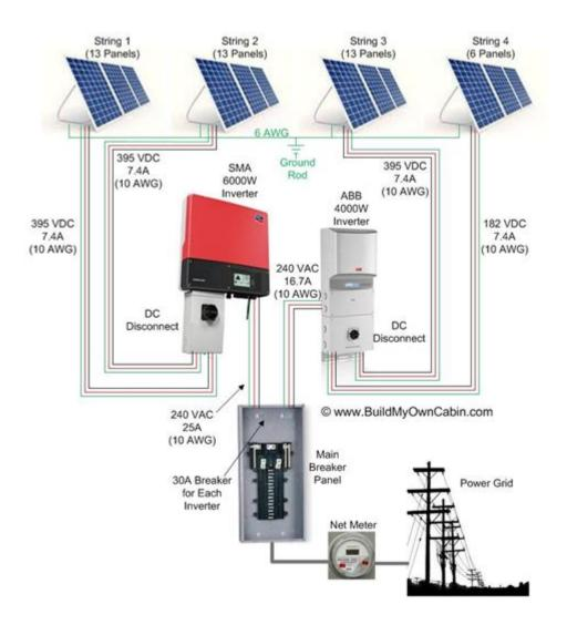
**Solar panels wiring diagram** is a crucial aspect of setting up a solar energy system. Understanding how to wire solar panels correctly can significantly influence the efficiency and safety of your solar installation. This article will guide you through the essentials of solar panel wiring, including types of wiring diagrams, components involved, and step-by-step instructions to help you visualize the entire process.
