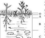
in soil has also been washed down to this layer. The partially weathered bedrock or **C horizon** is composed of broken up bedrock on top of the solid bedrock (parent material).
