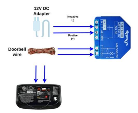
Shelly Plus 1 Wiring Diagram
