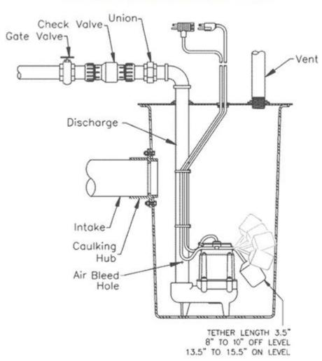
Sewage ejector pump installation diagram is an essential tool for homeowners and contractors alike who wish to understand the proper installation of sewage ejector systems. These systems are crucial for homes that have plumbing fixtures located below the level of the municipal sewer line. In this article, we will explore the components of a sewage ejector pump, the importance of proper installation, and provide a detailed guide on how to interpret a sewage ejector pump installation diagram.
