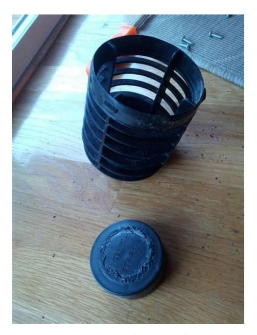
Shop vac ball float problem is a common issue faced by many users of wet/dry vacuums. The ball float mechanism is designed to prevent the vacuum from overflowing when the tank is full of liquid. However, problems can arise that may affect the efficiency of your shop vac. Understanding the ball float function, common issues, and solutions can help you maintain your equipment effectively and avoid costly repairs or replacements.
