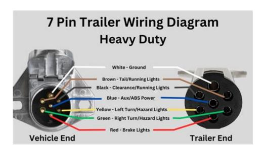
RV 7 Pin Wiring Diagram: Understanding the intricacies of RV wiring can be a daunting task for both novice and seasoned RV owners. The RV 7 pin wiring diagram is a crucial element in ensuring that your RV and tow vehicle communicate effectively, allowing for a seamless and safe towing experience. This article will delve into the details of the 7 pin wiring system, including its functions, wiring colors, common issues, and installation tips.
