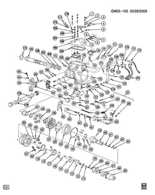
Roosa Master injection pump parts diagram serves as a crucial reference for mechanics and technicians working on diesel engines equipped with these pumps. Understanding the components of the Roosa Master injection pump is essential for performing maintenance, repairs, and troubleshooting effectively. This article delves into the parts of the Roosa Master injection pump, providing a comprehensive overview of its diagram, functionality, and the importance of each component.
