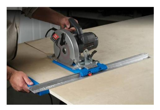
Rip guide for circular saw is an essential tool for anyone looking to achieve precise cuts in their woodworking projects. Whether you're a seasoned carpenter or a DIY enthusiast, mastering the use of a rip guide can significantly enhance the accuracy and efficiency of your work. In this detailed article, we will explore the importance of using a rip guide, how to set it up, and tips for making perfect rip cuts with your circular saw.
