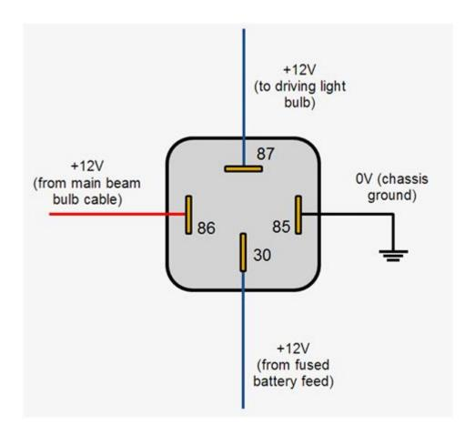
Relay 12 Volt Wiring Diagram is a crucial aspect of automotive and electrical system design, especially when it comes to controlling high-current devices with low-power signals. Relays serve as switches that allow a small current to control a larger one, making them essential for various applications, from automotive lighting to powering motors. This article will delve into the fundamentals of 12-volt relay wiring, its components, the wiring diagram, and practical applications.
