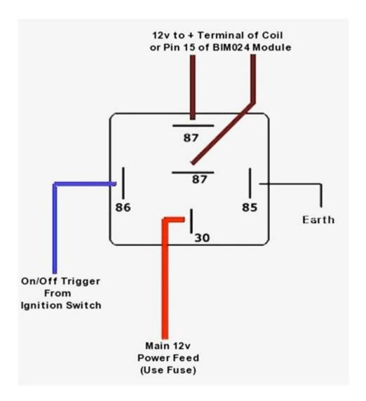
Relay wiring diagram 5 pin systems are essential components in various electrical applications, providing a means to control a higher power circuit using a lower power signal. Understanding how to wire a 5-pin relay can be crucial for anyone working with automotive or industrial electronics, home automation systems, or DIY projects. This article will delve into the intricacies of a 5-pin relay wiring diagram, including its components, applications, and step-by-step wiring instructions.
