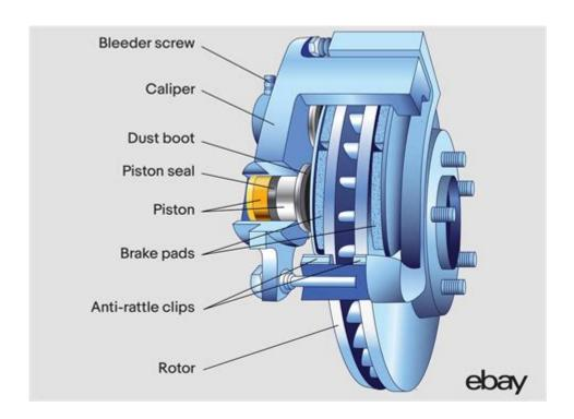
Rear brake caliper diagram is an essential tool for understanding the mechanics of a vehicle's braking system. The rear brake caliper plays a crucial role in ensuring safe and effective braking. This article will explore the components of a rear brake caliper, the function of each part, and how to interpret a typical rear brake caliper diagram.
