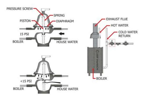
Pressure reducing valve installation diagram is an essential aspect of plumbing and hydraulic systems, ensuring that water pressure is maintained at safe and manageable levels. A pressure reducing valve (PRV) is crucial for any system where excessive pressure can lead to damage, inefficiency, or safety hazards. This article will provide an in-depth look at pressure reducing valves, their function, installation diagrams, and best practices for installation.
