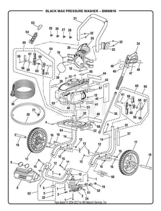
**Pressure washer pump diagram** is a crucial element for anyone interested in understanding how pressure washers operate. Knowing the inner workings of a pressure washer pump can empower users to maintain, troubleshoot, and optimize their equipment effectively. This article aims to provide a comprehensive overview of pressure washer pumps, including their components, functions, and how to read a pump diagram.
