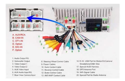
**podofo car stereo wiring diagram** is an essential tool for anyone looking to install or upgrade their car audio system. Understanding how to correctly interpret and utilize a wiring diagram can make all the difference between a seamless installation and a frustrating experience. This article will provide you with a comprehensive guide on podofo car stereo wiring diagrams, including what they are, how to read them, and tips for installation.
