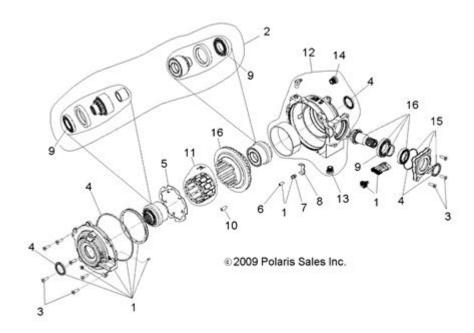
**Polaris RZR front differential parts diagram** is essential for understanding the inner workings of this important component of your Polaris RZR vehicle. The front differential plays a crucial role in delivering power to the front wheels, allowing for improved traction and handling in various terrains. This article will delve into the various parts of the front differential, their functions, and how to interpret a parts diagram for better maintenance and repair of your Polaris RZR.
