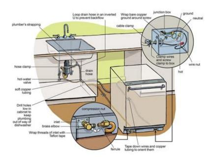
Plumbing under kitchen sink diagram with dishwasher installations can often look complex, but understanding the layout and components involved can simplify the process. In a typical kitchen, the plumbing under the sink is crucial for proper drainage, water supply, and appliance function. This article will provide a detailed overview of how to read and understand plumbing diagrams, specifically focusing on the integration of a dishwasher with the kitchen sink.
