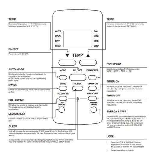
**Perfect Aire air conditioner remote control manual** is an essential guide for anyone who owns or operates a Perfect Aire air conditioning unit. Understanding how to effectively use the remote control can enhance your comfort and ensure efficient operation of your air conditioner. This article provides a comprehensive overview of the features, functions, and troubleshooting tips related to the Perfect Aire air conditioner remote control.
