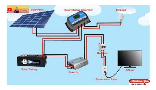
Off grid solar system wiring diagram is an essential aspect of designing and implementing a self-sufficient solar energy system. For many homeowners and businesses looking to reduce their reliance on traditional power grids, understanding how to properly wire an off-grid solar system is crucial. This article will provide a comprehensive overview of the components involved, the wiring process, and practical tips for creating an efficient off-grid solar setup.
