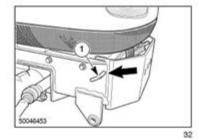
NOTE: Keep the latch mechanism free of dirt and debris, so the latch will operate properly.
