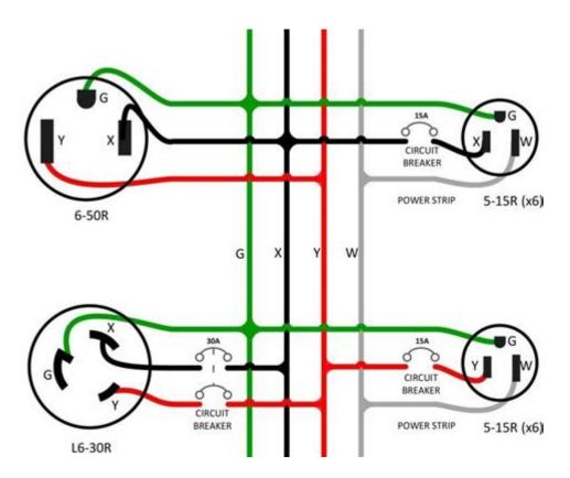
**NEMA L6-30R WIRING DIAGRAM** IS AN ESSENTIAL GUIDE FOR ANYONE WORKING WITH ELECTRICAL SYSTEMS THAT UTILIZE THIS SPECIFIC TYPE OF RECEPTACLE. THE NEMA L6-30R IS A LOCKING RECEPTACLE DESIGNED FOR 30-AMP, 250-VOLT APPLICATIONS. THIS TYPE OF RECEPTACLE IS COMMONLY USED IN INDUSTRIAL AND COMMERCIAL SETTINGS FOR POWERING HEAVY MACHINERY, WELDERS, AND OTHER HIGH-DEMAND ELECTRICAL EQUIPMENT. UNDERSTANDING HOW TO WIRE THIS RECEPTACLE SAFELY AND CORRECTLY IS CRUCIAL FOR BOTH FUNCTIONALITY AND SAFETY.
