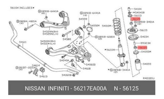
Nissan Xterra parts diagram is an essential resource for anyone looking to maintain or repair their vehicle. Understanding the various components of your Nissan Xterra can greatly simplify the process of sourcing parts and performing repairs. This article will delve into the various parts of the Nissan Xterra, how to access its parts diagram, and tips for maintenance and replacement.
