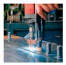
This provides the opportunity to weld process secured studs with a full-size diameter from 3 - 10mm with Drawn arc and from 4 - 7mm in Short cycle mode.
