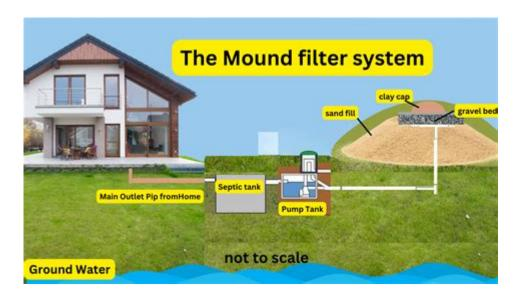
Mound septic system diagram is a crucial component in understanding how a mound septic system operates. These systems are a type of alternative wastewater treatment solution primarily designed for areas with poor drainage or a high water table. In this article, we will delve into the intricacies of mound septic systems, including their design, operation, advantages, disadvantages, and maintenance. We will also provide a detailed diagram to help visualize how these systems function.
