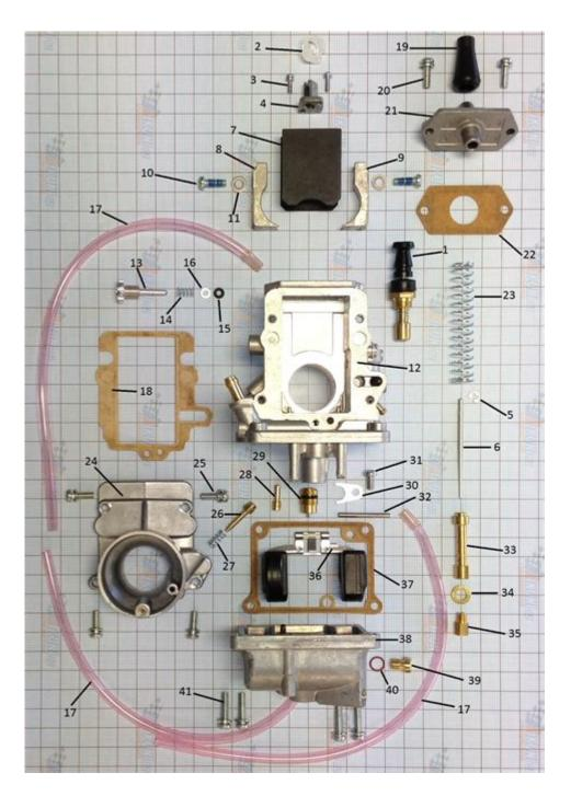
Mikuni carburetor parts diagram is an essential tool for anyone looking to understand the inner workings of these widely used components in various types of engines. Understanding the parts of a Mikuni carburetor can greatly enhance maintenance, troubleshooting, and tuning efforts. This article will delve into the various parts of a Mikuni carburetor, providing a detailed diagram and explanation of each component, along with maintenance tips and troubleshooting advice.
