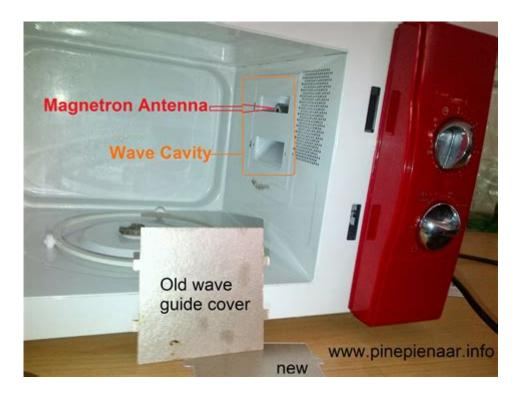
Microwave wave guide cover is a crucial component in the realm of microwave technology, particularly in domestic appliances like microwave ovens. It serves not only as a protective element but also plays a significant role in enhancing the efficiency and safety of microwave cooking. This article delves into the intricacies of microwave wave guide covers, their functions, design considerations, and maintenance tips, while also addressing common queries about their usage and effectiveness.
