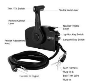
**Mercury throttle control diagram** is an essential concept for understanding how marine engines, particularly those manufactured by Mercury Marine, operate. The throttle control system is crucial for managing speed and power in outboard motors, inboard motors, and other marine applications. In this article, we will explore the components of the throttle control system, the significance of the throttle control diagram, how to interpret it, and maintenance tips to ensure optimal performance.
