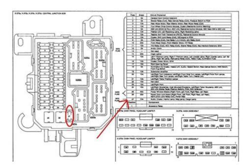
**Mazda 6 fuse box diagram** is an essential guide for owners and mechanics alike, providing critical information on the electrical system of the Mazda 6. Understanding the fuse box layout can help troubleshoot electrical issues, replace blown fuses, and maintain the vehicle's functionality. In this article, we will explore the fuse box diagrams specific to the Mazda 6, their locations, and how to interpret them effectively.
