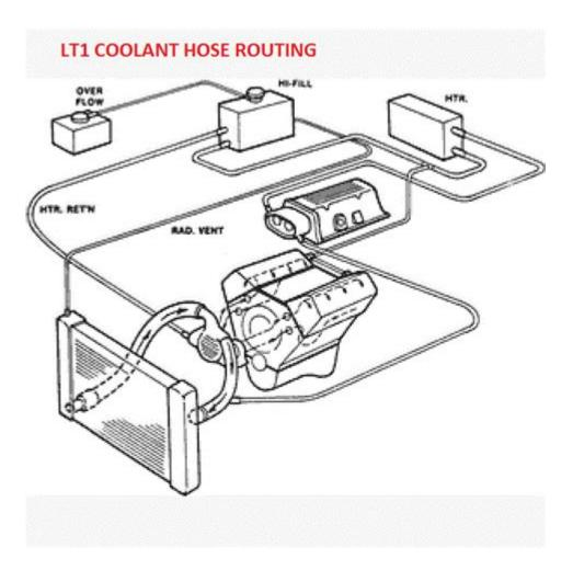
LT1 reverse flow cooling system diagram plays a crucial role in efficiently managing the thermal dynamics in high-performance engines, particularly the LT1 engine found in various Chevrolet models. This cooling system is designed to enhance performance by optimizing coolant flow and ensuring that the engine maintains an ideal operating temperature. In this article, we will explore the components, operation, advantages, and potential modifications related to the LT1 reverse flow cooling system.
