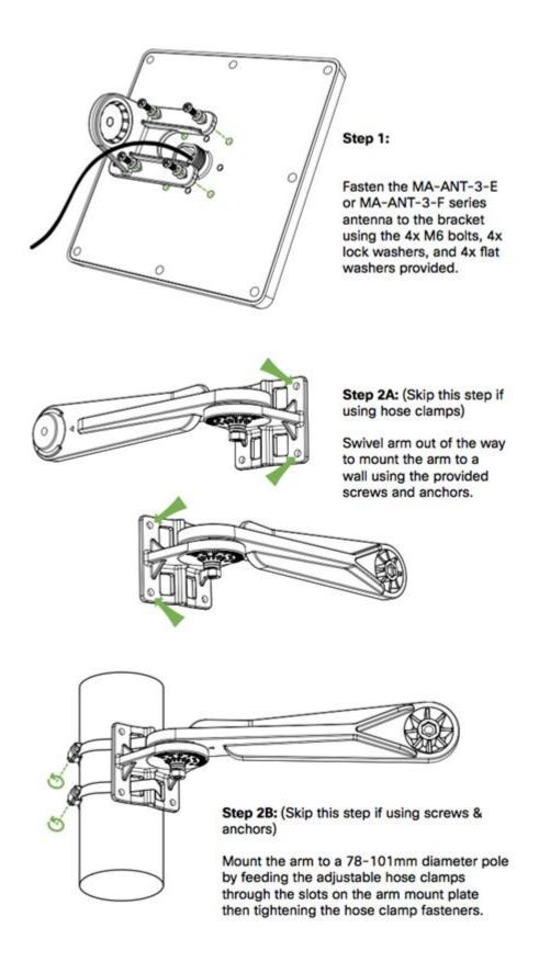
ma ant 25 installation guide: Installing the MA Ant 25 can be an exciting venture for both amateur and experienced radio enthusiasts. This high-performance antenna is designed to provide excellent
