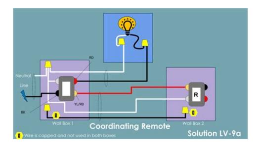
Leviton Smart Switch 3 Way Wiring Diagram is crucial for homeowners seeking to upgrade their lighting control systems. With the advent of smart home technology, replacing traditional switches with smart switches can significantly enhance convenience and efficiency. This article will provide a comprehensive guide on how to wire a Leviton smart switch in a three-way configuration, where two switches control a single light fixture from different locations.
