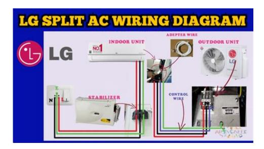
**LG mini split wiring diagram** is essential knowledge for anyone looking to install or troubleshoot an LG mini split air conditioning system. Understanding the wiring diagram can help you ensure that the unit operates efficiently and safely. In this article, we will explore the components of an LG mini split system, the significance of the wiring diagram, how to read and interpret it, installation guidelines, and common troubleshooting steps.
