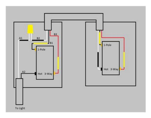
Legrand 3 Way Paddle Switch Wiring Diagram
