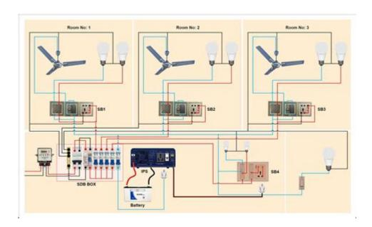
Lighting inverter wiring diagram is a critical topic for anyone looking to install or troubleshoot a lighting inverter system. An inverter converts direct current (DC) from batteries or solar panels into alternating current (AC), which powers lighting and other electrical appliances. Proper wiring is essential for the safe and efficient operation of an inverter. This article delves into the components, wiring diagrams, and tips for successfully implementing a lighting inverter system.
