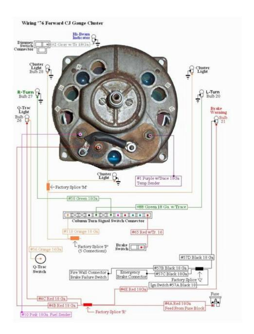
Jeep CJ5 wiring diagram is an essential resource for any Jeep enthusiast or owner looking to maintain, repair, or customize their vehicle's electrical system. Understanding the wiring diagram can help you troubleshoot issues, enhance your Jeep's performance, and ensure safety while driving. In this article, we'll explore the importance of having a wiring diagram, the components involved, and how to effectively read and use a Jeep CJ5 wiring diagram for your DIY projects.
