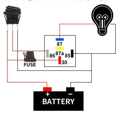
**jd1914 relay wiring diagram** is essential for understanding how to correctly wire relays in various electrical systems. Relays are critical components in automotive and industrial applications, allowing low-power circuits to control high-power devices. This article will delve into the specifics of the jd1914 relay wiring diagram, its applications, components, and troubleshooting tips to ensure effective and safe operation.
