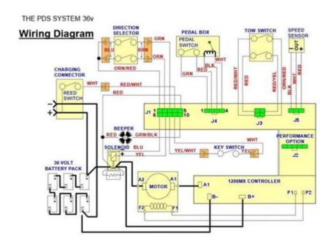
**Icon golf cart wiring diagram** is essential for any golf cart owner or technician who wants to understand the electrical system of their vehicle. Proper wiring is crucial for the performance and safety of your golf cart, ensuring that all electrical components function correctly. This article will explore the importance of wiring diagrams, how to read them, common wiring issues, and tips for maintaining your Icon golf cart's electrical system.
