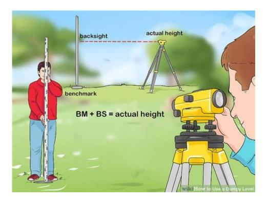
**How to use a dumpy level** is an essential skill for anyone involved in land surveying, construction, or landscaping. A dumpy level, also known as a builders' level or leveling instrument, is a type of optical level used to establish horizontal planes. This article will guide you through the process of using a dumpy level effectively, from understanding its components to setting it up and taking accurate measurements.
