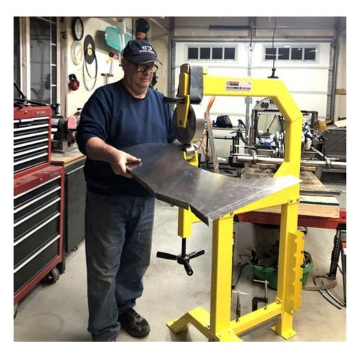
**How to use an English wheel** effectively requires understanding its components, techniques, and applications. This metalworking tool is primarily used for shaping and smoothing sheet metal, making it invaluable in automotive restoration, custom fabrication, and artistic metalworking. In this article, we will explore the parts of the English wheel, the setup process, and the techniques needed to master its use.
