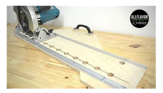
How to make a circular saw guide can significantly enhance your woodworking projects by ensuring precision and accuracy with every cut. A circular saw guide is an essential tool that helps you make straight cuts on various materials, including plywood, MDF, and solid wood. In this article, we will explore the step-by-step process of creating a circular saw guide, the materials needed, and tips for using it effectively.
