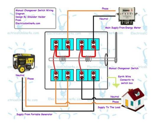
How to install a manual transfer switch is a critical skill for homeowners who want to ensure a safe and reliable power supply during outages. A manual transfer switch allows you to safely connect a portable generator to your home's electrical system, enabling you to power essential appliances when utility power is unavailable. This article will guide you through the process of selecting, installing, and using a manual transfer switch safely and effectively.
