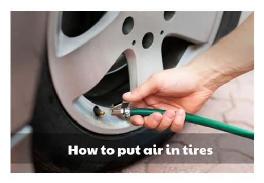
How to put air in tires is a crucial skill every car owner should master. Properly inflated tires not only enhance your vehicle's performance but also contribute to safety, fuel efficiency, and the longevity of the tires themselves. Over time, tires can lose air due to temperature changes, small punctures, or natural air permeation through the rubber. By regularly checking and maintaining the correct tire pressure, you can ensure a smoother, safer ride.
