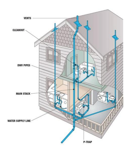
House plumbing system diagram is crucial for homeowners and builders alike to understand how water flows through a residence. A well-designed plumbing system ensures that the water supply is reliable and that waste is efficiently removed from the home. This article will explore the various components and layouts of a house plumbing system, providing insights into its functionality, common issues, and maintenance tips.
